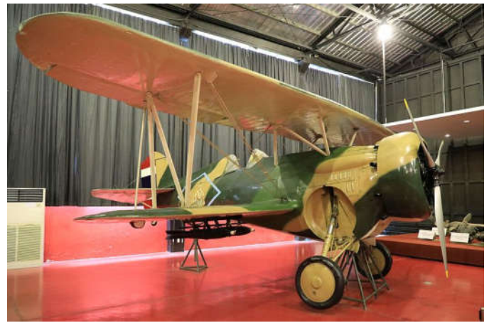
Above left , the last remaining Vought V-93S Corsair. This is a Thai version of the U.S. Navy's O3U-6 scout modified for ground attack with two additional forward firing machine guns. These entered service in 1934.
