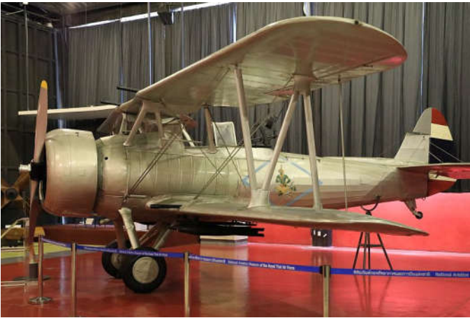
Above left , the last remaining Vought V-93S Corsair. This is a Thai version of the U.S. Navy's O3U-6 scout modified for ground attack with two additional forward firing machine guns. These entered service in 1934.
